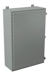
Wiegmann enclosure, NEMA 12/13,  $36 \times 24 \times 10$  in (HxWxD), wall mount, carbon steel, ANSI 61 gray, powder coat finish, single-door, (2) plated steel clamps, padlock hasp and staple.
