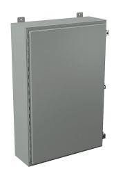
Wiegmann enclosure, NEMA 12/13, 36 x 24 x 8in (HxWxD), wall mount, carbon steel, ANSI 61 gray, powder coat finish, singledoor, (2) plated steel clamps, padlock hasp and staple.
