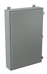
Wiegmann enclosure, NEMA 12/13, 36 x 24 x 6in (HxWxD), wall mount, carbon steel, ANSI 61 gray, powder coat finish, singledoor, (2) plated steel clamps, padlock hasp and staple.
