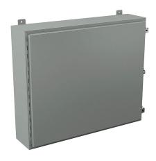
Wiegmann enclosure, NEMA 12/13, 30 x 36 x 8in (HxWxD), wall mount, carbon steel, ANSI 61 gray, powder coat finish, singledoor, (2) plated steel clamps, padlock hasp and staple.
