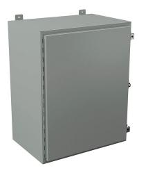
Wiegmann enclosure, NEMA 12/13,  $30 \times 24 \times 16$  in (HxWxD), wall mount, carbon steel, ANSI 61 gray, powder coat finish, single-door, (2) plated steel clamps, padlock hasp and staple.
