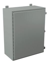
Wiegmann enclosure, NEMA 12/13, 30 x 24 x 12in (HxWxD), wall mount, carbon steel, ANSI 61 gray, powder coat finish, single-door, (2) plated steel clamps, padlock hasp and staple.
