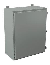
Wiegmann enclosure, NEMA 12/13, 30 x 24 x 12in (HxWxD), wall mount, carbon steel, ANSI 61 gray, powder coat finish, singledoor, (2) plated steel clamps, padlock hasp and staple.
