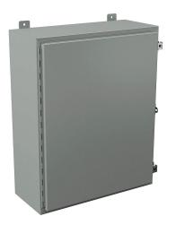
Wiegmann enclosure, NEMA 12/13, 30 x 24 x 10in (HxWxD), wall mount, carbon steel, ANSI 61 gray, powder coat finish, singledoor, (2) plated steel clamps, padlock hasp and staple.
