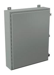
Wiegmann enclosure, NEMA 12/13, 30 x 24 x 6in (HxWxD), wall mount, carbon steel, ANSI 61 gray, powder coat finish, singledoor, (2) plated steel clamps, padlock hasp and staple.
