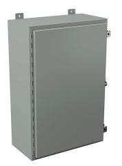
Wiegmann enclosure, NEMA 12/13, 30 x 20 x 10in (HxWxD), wall mount, carbon steel, ANSI 61 gray, powder coat finish, single-door, (2) plated steel clamps, padlock hasp and staple.
