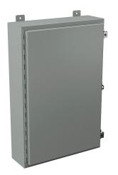
Wiegmann enclosure, NEMA 12/13, 30 x 20 x 6in (HxWxD), wall mount, carbon steel, ANSI 61 gray, powder coat finish, single-door, (2) plated steel clamps, padlock hasp and staple.
