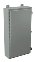
Wiegmann enclosure, NEMA 12/13, 30 x 16 x 6in (HxWxD), wall mount, carbon steel, ANSI 61 gray, powder coat finish, singledoor, (2) plated steel clamps, padlock hasp and staple.
