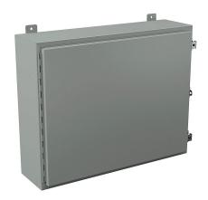
Wiegmann enclosure, NEMA 12/13, 24 x 30 x 8in (HxWxD), wall mount, carbon steel, ANSI 61 gray, powder coat finish, singledoor, (2) plated steel clamps, padlock hasp and staple.
