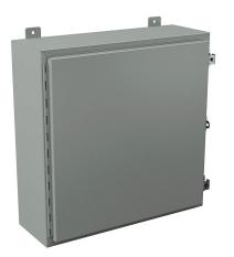
Wiegmann enclosure, NEMA 12/13, 24 x 24 x 8in (HxWxD), wall mount, carbon steel, ANSI 61 gray, powder coat finish, single-door, (2) plated steel clamps, padlock hasp and staple.
