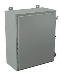
Wiegmann enclosure, NEMA 12/13, 24 x 20 x 10in (HxWxD), wall mount, carbon steel, ANSI 61 gray, powder coat finish, singledoor, (2) plated steel clamps, padlock hasp and staple.
