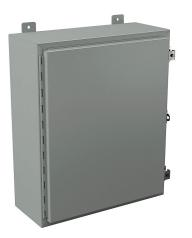
Wiegmann enclosure, NEMA 12/13, 24 x 20 x 8in (HxWxD), wall mount, carbon steel, ANSI 61 gray, powder coat finish, single-door, (2) plated steel clamps, padlock hasp and staple.
