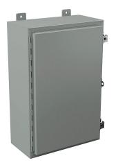
Wiegmann enclosure, NEMA 12/13, 24 x 16 x 8in (HxWxD), wall mount, carbon steel, ANSI 61 gray, powder coat finish, single-door, (2) plated steel clamps, padlock hasp and staple.
