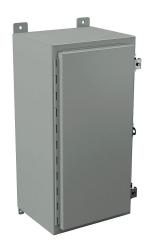
Wiegmann enclosure, NEMA 12/13, 24 x 12 x 10in (HxWxD), wall mount, carbon steel, ANSI 61 gray, powder coat finish, singledoor, (2) plated steel clamps, padlock hasp and staple.
