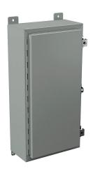
Wiegmann enclosure, NEMA 12/13, 24 x 12 x 6in (HxWxD), wall mount, carbon steel, ANSI 61 gray, powder coat finish, singledoor, (2) plated steel clamps, padlock hasp and staple.
