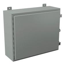
Wiegmann enclosure, NEMA 12/13, 20 x 24 x 8in (HxWxD), wall mount, carbon steel, ANSI 61 gray, powder coat finish, single-door, (2) plated steel clamps, padlock hasp and staple.
