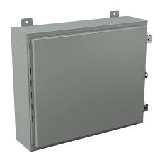
Wiegmann enclosure, NEMA 12/13, 20 x 24 x 6in (HxWxD), wall mount, carbon steel, ANSI 61 gray, powder coat finish, singledoor, (2) plated steel clamps, padlock hasp and staple.
