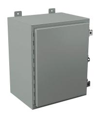
Wiegmann enclosure, NEMA 12/13, 20 x 16 x 12in (HxWxD), wall mount, carbon steel, ANSI 61 gray, powder coat finish, singledoor, (2) plated steel clamps, padlock hasp and staple.
