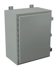
Wiegmann enclosure, NEMA 12/13, 20 x 16 x 10in (HxWxD), wall mount, carbon steel, ANSI 61 gray, powder coat finish, singledoor, (2) plated steel clamps, padlock hasp and staple.
