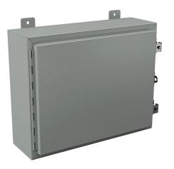
Wiegmann enclosure, NEMA 12/13, 16 x 20 x 6in (HxWxD), wall mount, carbon steel, ANSI 61 gray, powder coat finish, single-door, (2) plated steel clamps, padlock hasp and staple.
