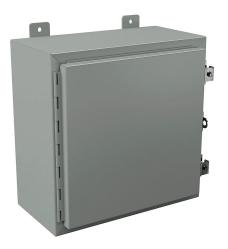
Wiegmann enclosure, NEMA 12/13, 16 x 16 x 8in (HxWxD), wall mount, carbon steel, ANSI 61 gray, powder coat finish, single-door, (2) plated steel clamps, padlock hasp and staple.
