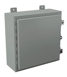
Wiegmann enclosure, NEMA 12/13, 16 x 16 x 6in (HxWxD), wall mount, carbon steel, ANSI 61 gray, powder coat finish, singledoor, (2) plated steel clamps, padlock hasp and staple.
