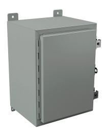
Wiegmann enclosure, NEMA 12/13, 16 x 12 x 10in (HxWxD), wall mount, carbon steel, ANSI 61 gray, powder coat finish, singledoor, (2) plated steel clamps, padlock hasp and staple.
