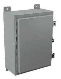
Wiegmann enclosure, NEMA 12/13, 16 x 12 x 6in (HxWxD), wall mount, carbon steel, ANSI 61 gray, powder coat finish, single-door, (2) plated steel clamps, padlock hasp and staple.
