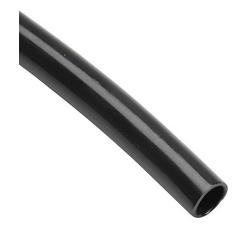
NITRA pneumatic tubing, nylon 12, black, 10mm outside diameter, 5/16in (8mm) inside diameter, 100ft package.
