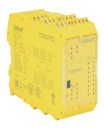
ReeR MOSAIC standalone safety controller, 24 VDC, (16) digital safety input(s), (4) EDM/(re)start input(s), (4) pair OSSD safety output(s), pluggable screw terminals.
