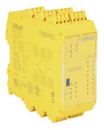
ReeR MOSAIC standalone safety controller, 24 VDC, (16) digital safety input(s), (4) EDM/(re)start input(s), (4) pair OSSD safety output(s), push-in cage clamp.
