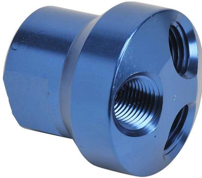
NITRA pneumatic valve manifold, aluminum, blue, round, 500 psi maximum operating pressure, (3) stations, (1) 1/4in female NPT inlet(s), (3) 1/4in female NPT outlet(s).
