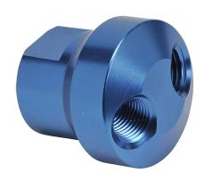
NITRA pneumatic valve manifold, aluminum, round, 500 psi maximum operating pressure, (2) stations, (1) 1/4in female NPT inlet(s), (2) 1/4in female NPT outlet(s).
