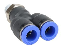
NITRA pneumatic push-to-connect fitting, Y, rotating, thermoplastic (PBT) body, nickel-plated brass threads, thread sealant, (1) R1/8 male BSPT to (2) 5/16in (8mm) push-to-connect. Package of 5.
