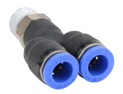
NITRA pneumatic push-to-connect fitting, Y, rotating, thermoplastic (PBT) body, nickel-plated brass threads, thread sealant, (1) R1/4 male BSPT to (2) 5/16in (8mm) push-to-connect. Package of 5.
