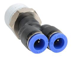
NITRA pneumatic push-to-connect fitting, Y, rotating, thermoplastic (PBT) body, nickel-plated brass threads, thread sealant, (1) R1/2 male BSPT to (2) 5/16in (8mm) push-to-connect. Package of 5.
