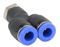
NITRA pneumatic push-to-connect fitting, Y, rotating, thermoplastic (PBT) body, nickel-plated brass threads, thread sealant, (1) M5 x 0.8 male ISO to (2) 6mm push-to-connect. Package of 5.
