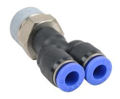
NITRA pneumatic push-to-connect fitting, Y, rotating, thermoplastic (PBT) body, nickel-plated brass threads, thread sealant, (1) R3/8 male BSPT to (2) 6mm push-to-connect. Package of 5.
