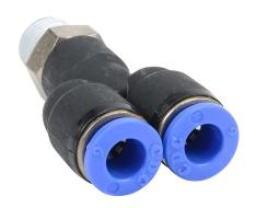
NITRA pneumatic push-to-connect fitting, Y, rotating, thermoplastic (PBT) body, nickel-plated brass threads, thread sealant, (1) R1/8 male BSPT to (2) 6mm push-to-connect. Package of 5.
