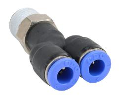
NITRA pneumatic push-to-connect fitting, Y, rotating, thermoplastic (PBT) body, nickel-plated brass threads, thread sealant, (1) R1/4 male BSPT to (2) 6mm push-to-connect. Package of 5.
