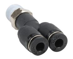
NITRA pneumatic push-to-connect fitting, Y, rotating, thermoplastic (PBT) body, nickel-plated brass threads, thread sealant, (1) 1/8in male NPT to (2) 5/32in (4mm) push-to-connect. Package of 5.
