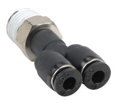
NITRA pneumatic push-to-connect fitting, Y, rotating, thermoplastic (PBT) body, nickel-plated brass threads, thread sealant, (1) 1/4in male NPT to (2) 5/32in (4mm) push-to-connect. Package of 5.
