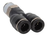
NITRA pneumatic push-to-connect fitting, Y, rotating, thermoplastic (PBT) body, nickel-plated brass threads, thread sealant, (1) 1/4in male NPT to (2) 5/16in (8mm) push-to-connect. Package of 5.
