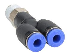
NITRA pneumatic push-to-connect fitting, Y, rotating, thermoplastic (PBT) body, nickel-plated brass threads, thread sealant, (1) R1/8 male BSPT to (2) 5/32in (4mm) push-to-connect. Package of 5.
