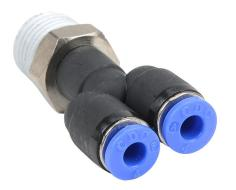
NITRA pneumatic push-to-connect fitting, Y, rotating, thermoplastic (PBT) body, nickel-plated brass threads, thread sealant, (1) R1/4 male BSPT to (2) 5/32in (4mm) push-to-connect. Package of 5.
