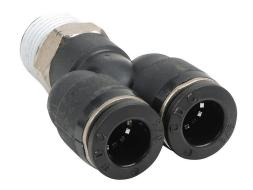
NITRA pneumatic push-to-connect fitting, male, Y, rotating, thermoplastic (PBT) body, nickel-plated brass threads, (2) 3/8in tube to 3/8in NPT connection(s). Package of 5.
