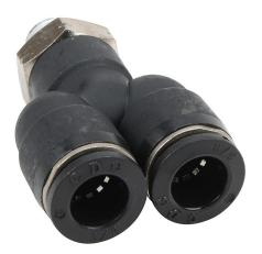
NITRA pneumatic push-to-connect fitting, Y, rotating, thermoplastic (PBT) body, nickel-plated brass threads, thread sealant, (2) 3/8in push-to-connect to (1) 1/8in male NPT. Package of 5.
