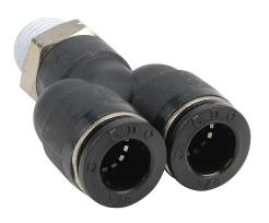
NITRA pneumatic push-to-connect fitting, Y, rotating, thermoplastic (PBT) body, nickel-plated brass threads, thread sealant, (1) 1/4in male NPT to (2) 3/8in push-to-connect. Package of 5.
