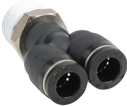
NITRA pneumatic push-to-connect fitting, Y, rotating, thermoplastic (PBT) body, nickel-plated brass threads, thread sealant, (1) 1/2in male NPT to (2) 3/8in push-to-connect. Package of 5.
