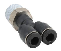
NITRA pneumatic push-to-connect fitting, Y, rotating, thermoplastic (PBT) body, nickel-plated brass threads, thread sealant, (1) 3/8in male NPT to (2) 1/4in push-to-connect. Package of 5.
