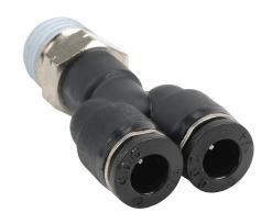
NITRA pneumatic push-to-connect fitting, Y, rotating, thermoplastic (PBT) body, nickel-plated brass threads, thread sealant, (1) 1/4in male NPT to (2) 1/4in push-to-connect. Package of 5.
